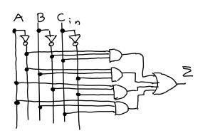
(5) When circuit: are already in the AND-OR config., it is straight-forward to turn them into circuits which use only NAND gates.
